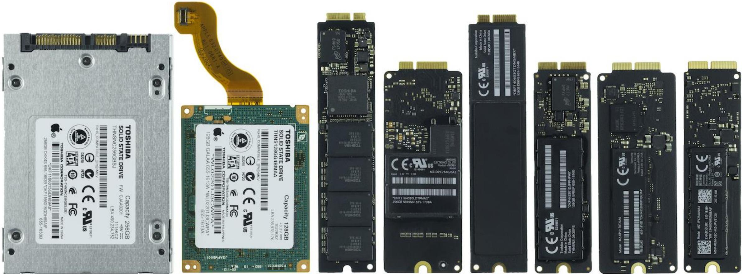
Gen. 1 SSD, Gen. 2B, Gen. 2A, Gen. 3A (comparable to Gen. 4A and Gen. 4C),
