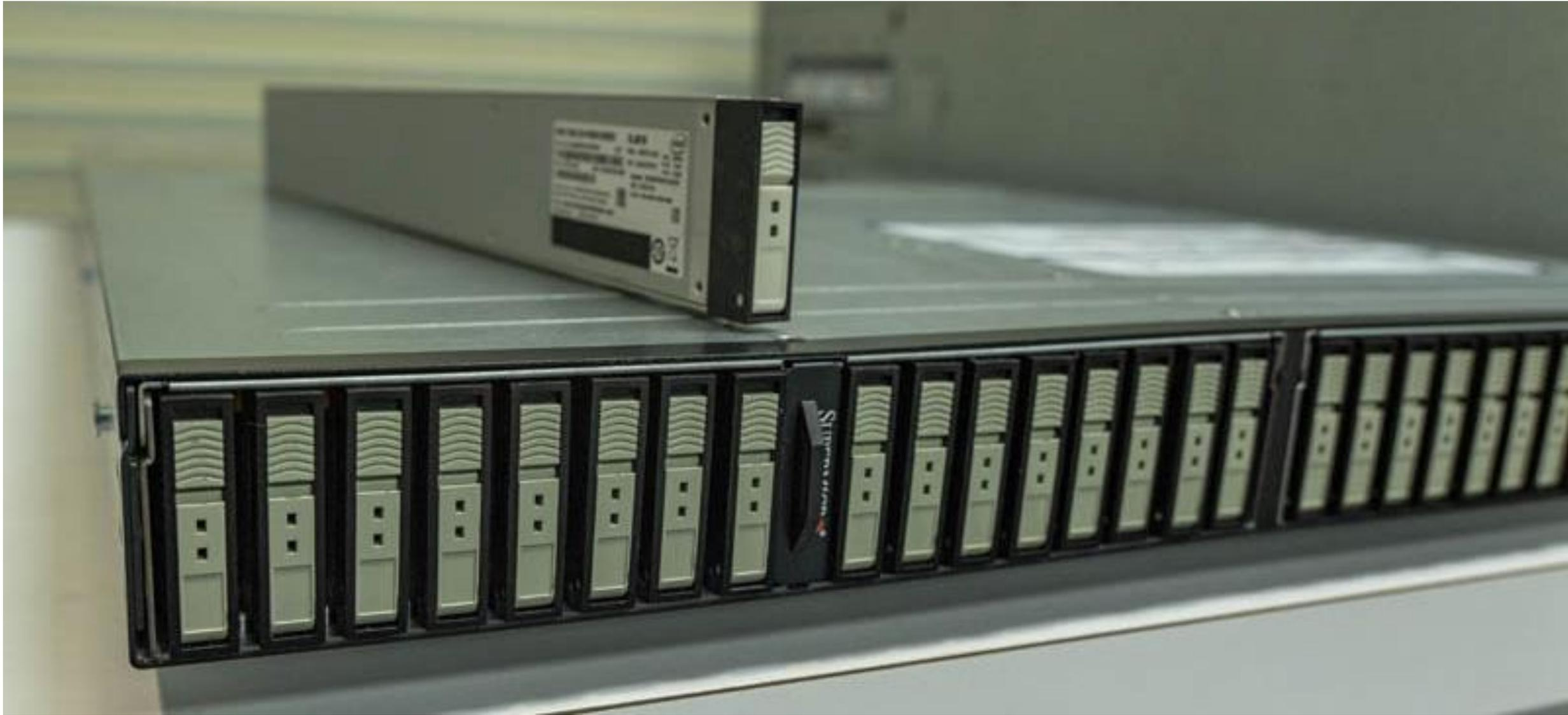
Supermicro SSG 1029P NEL32R With 15TB Intel EDSFF SSD On Top
